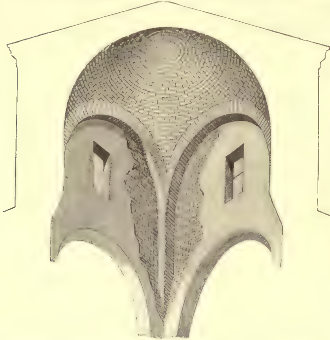
Fig. 39.—Ravenna. Mausoleum of Galla Placidia. Construction of the Cupola (about 440).
